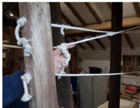
Re-roping the sack hoist control system
